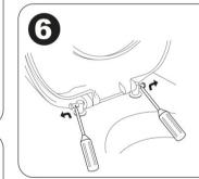
In case of improper installation, remove the hinge pin in both side and reverse the procedure by following back to step 5 again.
