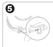
Assemble the seat & cover into Hinge body by insert Hinge pin through to both side of Hinge body set (see the picture). Re-check all over again, to see whether the seat & cover are fit properly into the toilet seat.
